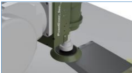
Slag removal for thick plate/gas cutting
