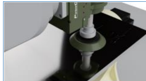
Scratch removal/polishing of steel plate
