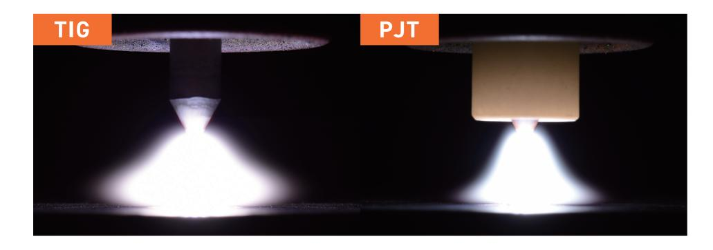
Workpiece: SUSt3.0mm | tanning weld
