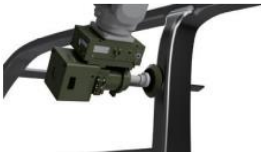
Automotive B-pillar brazing polishing
