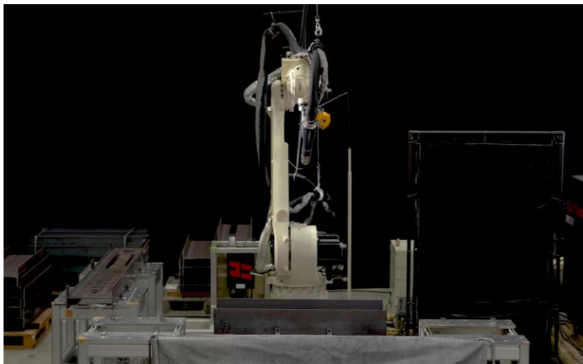
6.5 mm thick H-beam: High-speed cutting
